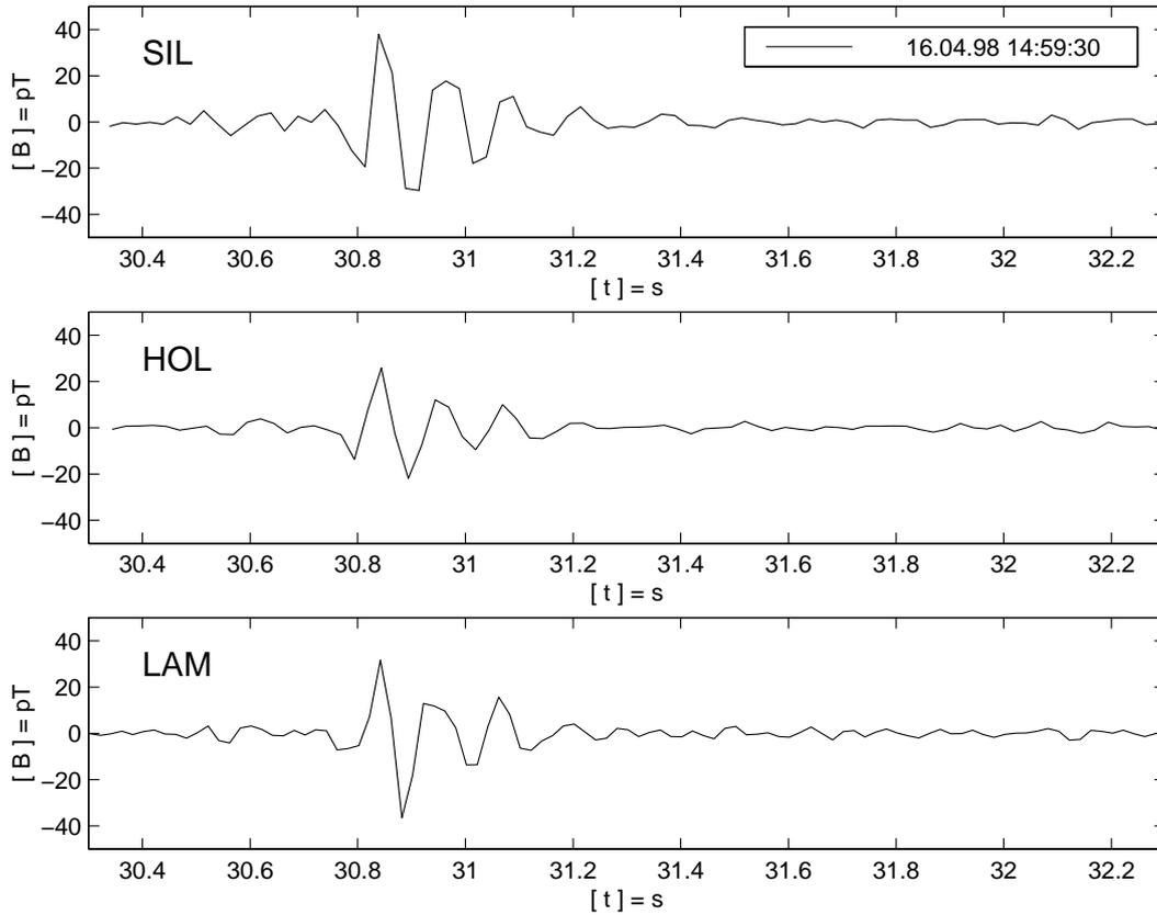
Temporal synchronisation of the stations is ensured with the aid of GPS satellites. Through cross-correlation of these three time series, lightning can then be located with an accuracy of several 100 km with the aid of spherical geometry. Fig.6, for instance, shows the result of such measurements for one month, which can be used for the study of global thunderstorm activity [5]. A global network for monitoring of lightning is being developed as a warning system for air traffic.
