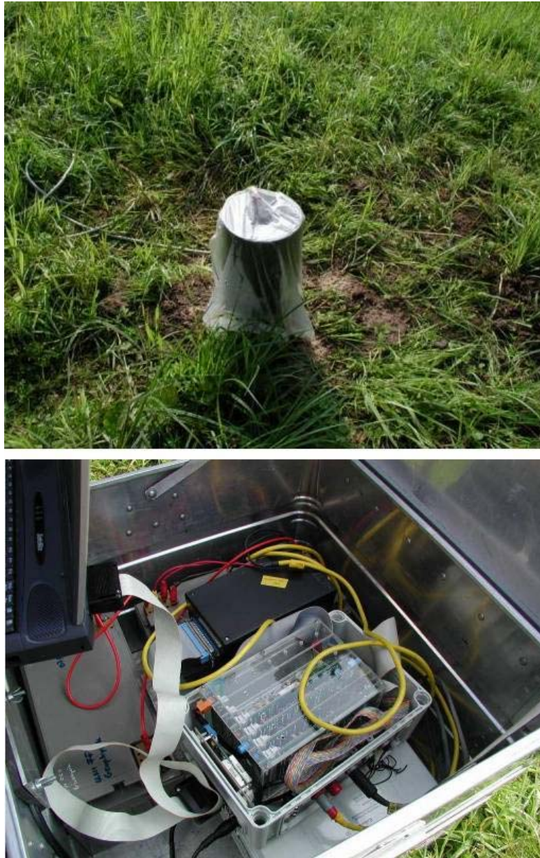
Fig. 4: Vertically placed coil for the measurement of the vertical component of the Schumann resonance (above) and electronics box for the detection and storage of the time signal (below). Because Schumann resonance must be measured far away from technical disturbances, the entire electronics is operated in the open with batteries.
